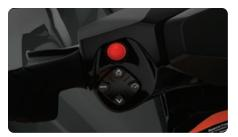
VTS<sup>™</sup> (Variable Trim System) Provides handlebar-activated settings so riders can easily find the ideal trim for varying conditions.
