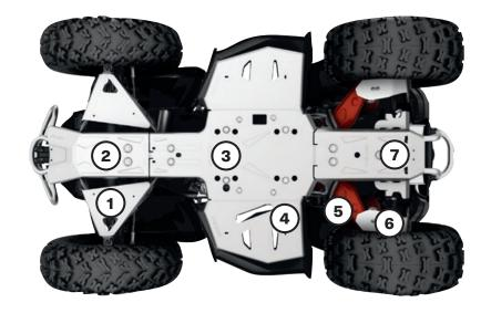
For ultimate durability and strength, all our Aluminum Skid Plates are made with 3/16" (4.5 mm) thick High Strength 5052 H32 Aluminum.
